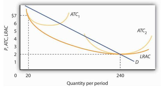
A firm with falling LRAC throughout the range of outputs relevant to existing demand (D) will monopolize the industry. Here, one firm operating with a large plant ( $ATC_2$ ) produces 240 units of output at a lower cost than the \$7 cost per unit of the 12 firms operating at a smaller scale ( $ATC_1$ ), and producing 20 units of output each.
