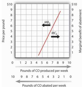
The marginal cost of the first few units of emissions is zero and then rises once emissions begin to harm people. That is the point at which the air becomes a scarce resource. Read from left to right the curve gives the marginal cost of emissions ( $MC_E$ ). Read from right to left, the curve gives the marginal benefit of abatement ( $MB_A$ ).
