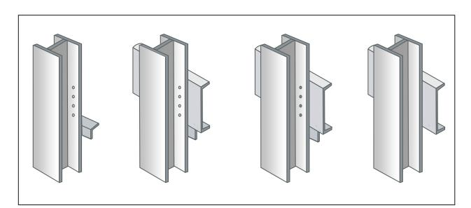
Drawing of Mies van der Rohe, Plug weld procedure: connection prepared, beam placed, plug weld, connection finished.
