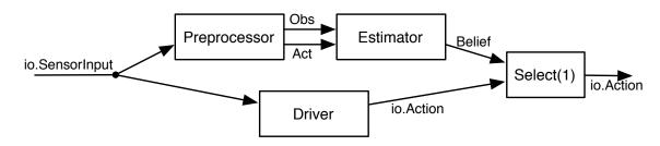
The Driver, PreProcessor and Select state machine classes are already implemented. The Driver machine generates instances of io.Action that make the robot move forward; the Select(1) machine takes tuples (or lists) of values as input and always returns the second element of the tuple as output. The robot knows the ideal readings for each of the possible discrete locations it might be in, but doesn't know where it is initially; the goal of the state estimation process
