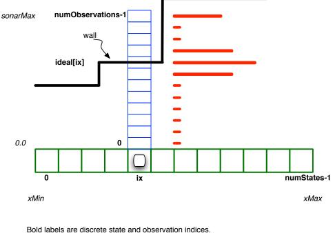
Bold labels are discrete state and observation indices. Italic labels are real-valued robot locations or sonar readings. Dark line is actual location of a wall. Green boxes are possible discrete robot locations. Blue boxes are possible discrete sonar readings. Red bars indicate the distribution observationDistribution(ix). The file lineLocalizeSkeleton.py contains the following skeleton of a procedure that should construct and return the appropriate ssm.StochasticSM model. The parameters are:
