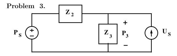
Figure 2: An acoustic circuit consisting of a pressure source, a volume velocity source and two impedances. All pressures and volume velocities are assumed to have the same  $e^{st}$  time dependence.
