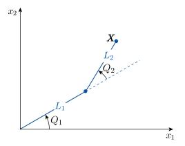
Figure 2: Schematic of robot arm: end effector  $\boldsymbol{X} = (X_1 \ X_2)^{\mathrm{T}}$  and joint angles  $\boldsymbol{Q} = (Q_1 \ Q_2)^{\mathrm{T}}$ .
