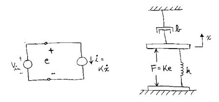
Here, the piezoelectric actuator is modeled internally as a dependent force source F(t) in parallel with a spring k. The force depends linearly upon the input voltage as F(t) = Ke(t), where K is a scale factor with units of N/V. The spring k models the internal stiffness of the piezoelectric actuator. The force F is applied to the massless upper plate which connects the damper and spring.
