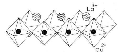
Due to the distortion of the oxygen octahedra, the highest energy d orbital on the copper site is described by a single  $d_{x^2-y^2}$  orbital with energy  $E_d$ . We use the approximation of retaining the degenerate  $p_x, p_y$  with orbitals at energy  $E_p$  on the oxygen sites.
