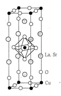
FIG. 1. Crystal structure of  $La_{2-x}Sr_xCuO_4$  (T phase). Taken from Almasan and Maple (1991).
