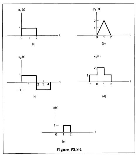
(b) Determine and sketch the response of the system considered in part (a) to the input  $x_3(t)$  shown in Figure P3.8-1(d).
