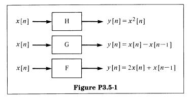
The systems in Figures P3.5-2 to P3.5-7 are formed by parallel and cascade combination of H, G, and F. By expressing the output y[n] in terms of the input x[n], determine which of the systems are equivalent.
