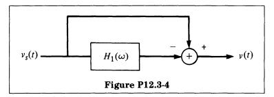
Sketch  $V(\omega)/V_s(\omega)$ . What is the corresponding cutoff frequency?
