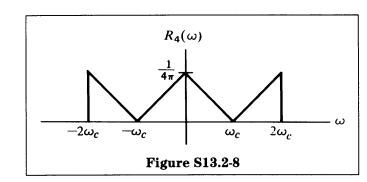
$R_4(\omega)$  is given by shifting  $R_3(\omega)$  up and down by  $\omega_c$  and dividing by 2. See Figure S13.2-8.
