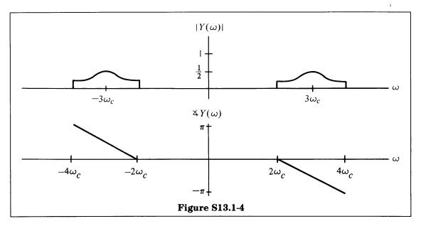
(e) Since the phase terms are different in parts (c) and (d), we cannot just add spectra. We need to convert  $\cos 3\omega_c t + \sin 3\omega_c t$  into the form  $A \cos(3\omega_c t + \theta)$ . Note
