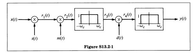
By the modulation property,  $R_1(\omega)$ , the Fourier transform of  $r_1(t)$ , is
