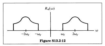
After filtering, y(t) = 0 since  $R_4(\omega)$  has no energy from  $-\omega_c$  to  $\omega_c$ . (e) For this part, let us calculate  $R_2(\omega)$  explicitly.
