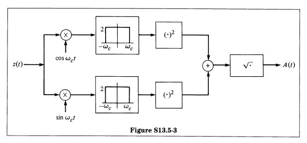
Note that to be able to recover A(t) in this way, the Fourier transform of A(t) must be zero for  $\omega > |\omega_c|$  and A(t) > 0. Also note that we are implicitly assuming that A(t) is a real signal.
