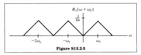
Similarly, modulating by  $e^{-j\omega_c t}$  yields  $R_1(\omega + \omega_c)$  as shown in Figure S13.2-5.
