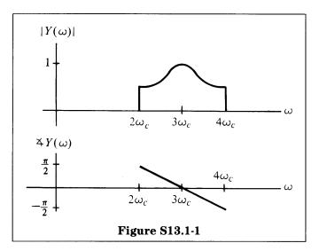
(b) Since  $e^{j3\omega_c+j\pi/2} = e^{j\pi/2}e^{j3\omega_c t}$ , we are modulating the same carrier as in part (a) except that we multiply the result by  $e^{j\pi/2}$ . Thus
