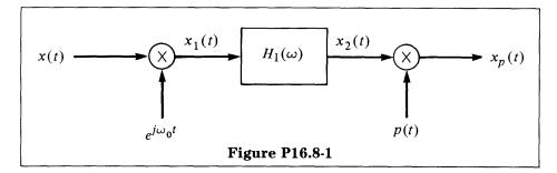
With x(t) real and with  $X(\omega)$  nonzero only for  $\omega_1 < |\omega| < \omega_2$ , the modulating frequency  $\omega_0$  is chosen as  $\omega_0 = \frac{1}{2}(\omega_1 + \omega_2)$ , and the lowpass filter  $H_1(\omega)$  has cutoff frequency  $\frac{1}{2}(\omega_2 - \omega_1)$ .
