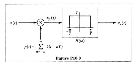
The sampling period T is 1 ms, and x(t) is a sinusoidal signal of the form  $x(t) = \cos(2\pi f_0 t + \theta)$ . For each of the following choices of  $f_0$  and  $\theta$ , determine  $x_r(t)$ .
