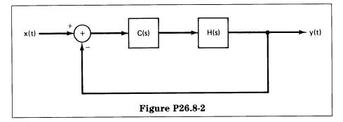
(c) Show that the system of Figure P26.8-2 can be stabilized if C(s) is a proportional plus derivative system:
