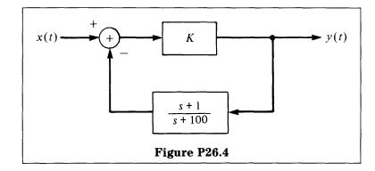
Find the closed-loop poles and zeros of this system for the following values of K:
