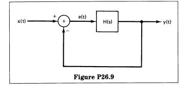
(a) Use the final value theorem (Section 9.5.9 of the text) to show that a Type 1 feedback system can track a step, i.e., that
