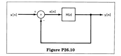
(b) More generally, consider the feedback system of Figure P26.10 and assume that the closed-loop system is stable. Suppose that H(z) has a pole at z = 1. Show that the system can track a unit step. [Hint: Express the transform E(z) of e[n] in terms of H(z) and the transform of u[n]; explain why all the poles of E(z) are inside the unit circle.]
