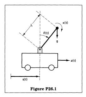
Our goal in this problem is to analyze the dynamics of the inverted pendulum and more specifically to investigate the problem of balancing the pendulum by judicious choice of the cart acceleration a(t). The differential equation relating  $\theta(t)$ , a(t), and x(t) is
