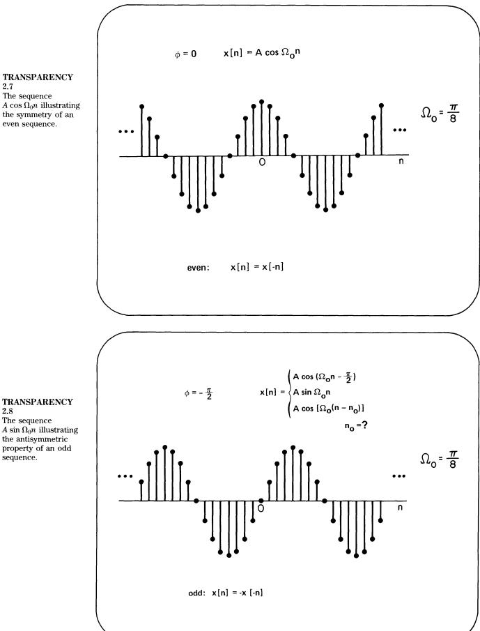
TRANSPARENCY 2.8 The sequence  $A \sin \Omega_0 n$  illustrating the antisymmetric property of an odd sequence.
